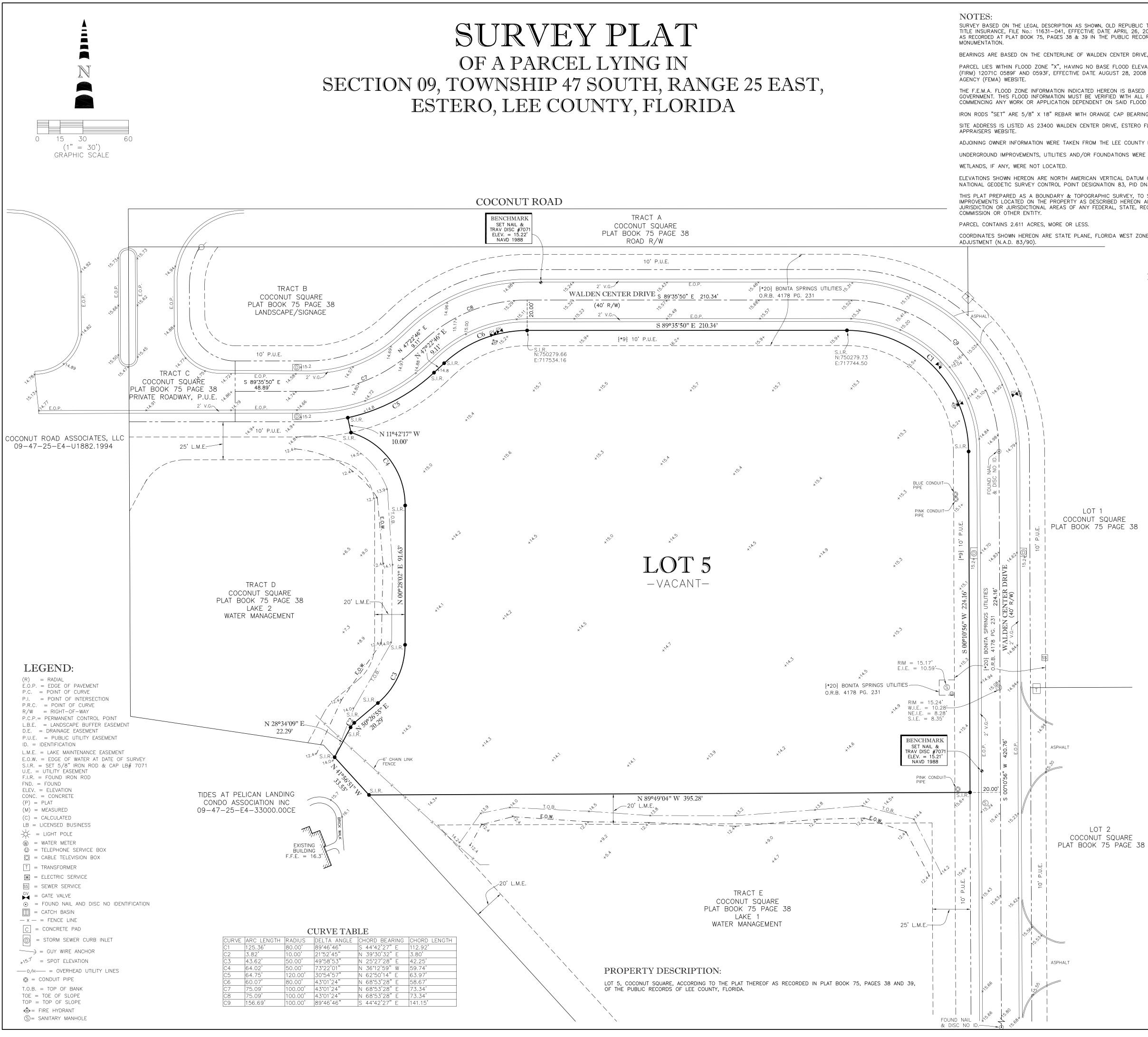
BEARINGS ARE BASED ON THE CENTERLINE OF WALDEN CENTER DRIVE, AS BEARING S89'35'50"E. PARCEL LIES WITHIN FLOOD ZONE "X", HAVING NO BASE FLOOD ELEVATION, PER FLOOD INSURANCE RATE MAP (FIRM) 12071C 0589F AND 0593F, EFFECTIVE DATE AUGUST 28, 2008 AND THE FEDERAL EMERGENCY MANAGEMENT
