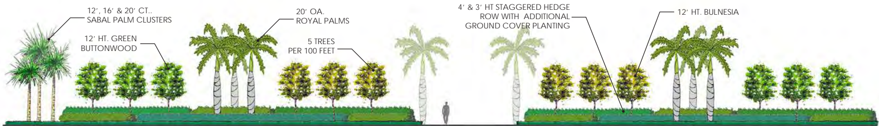
CORKSCREW BUFFER ELEVATION (20' TYPE D BUFFER - ENHANCED)
