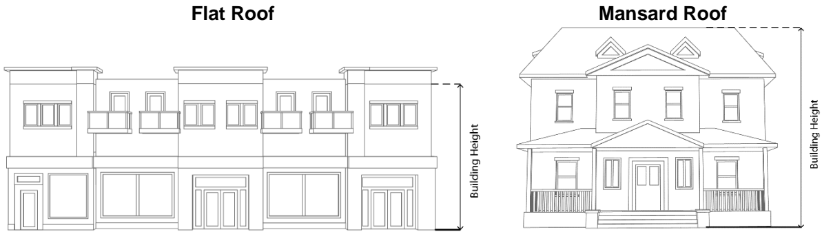
Figure 10-301.C-1: Flat and Mansard Roof Building Height Measurement
