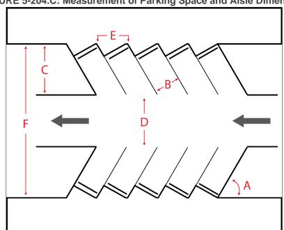
FIGURE 5-204.C: Measurement of Parking Space and Aisle Dimension
