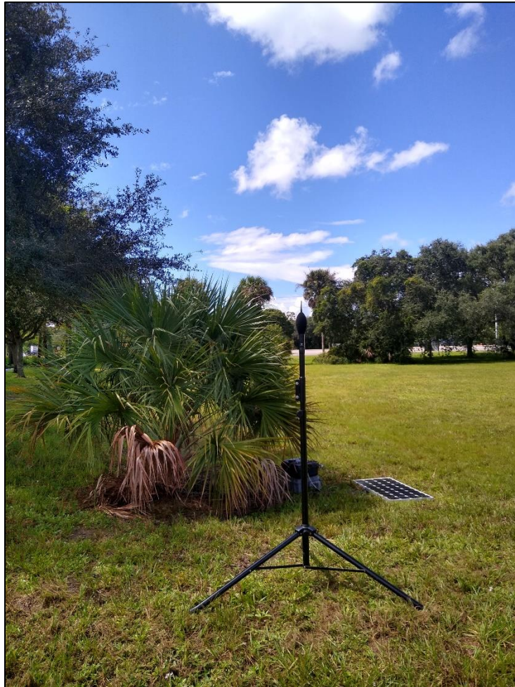
Figure 3. Measurement microphone used for long-term acoustical measurements at the project site.
