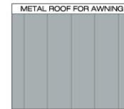
METAL ROOF FOR AWNING STANDING SEAM METAL PANEL FOR THE AWNINGS - COLOR "DOVE GRAY"
