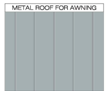
METAL ROOF FOR AWNING STANDING SEAM METAL PANEL FOR THE THE AWNINGS - COLOR "DOVE GRAY"
