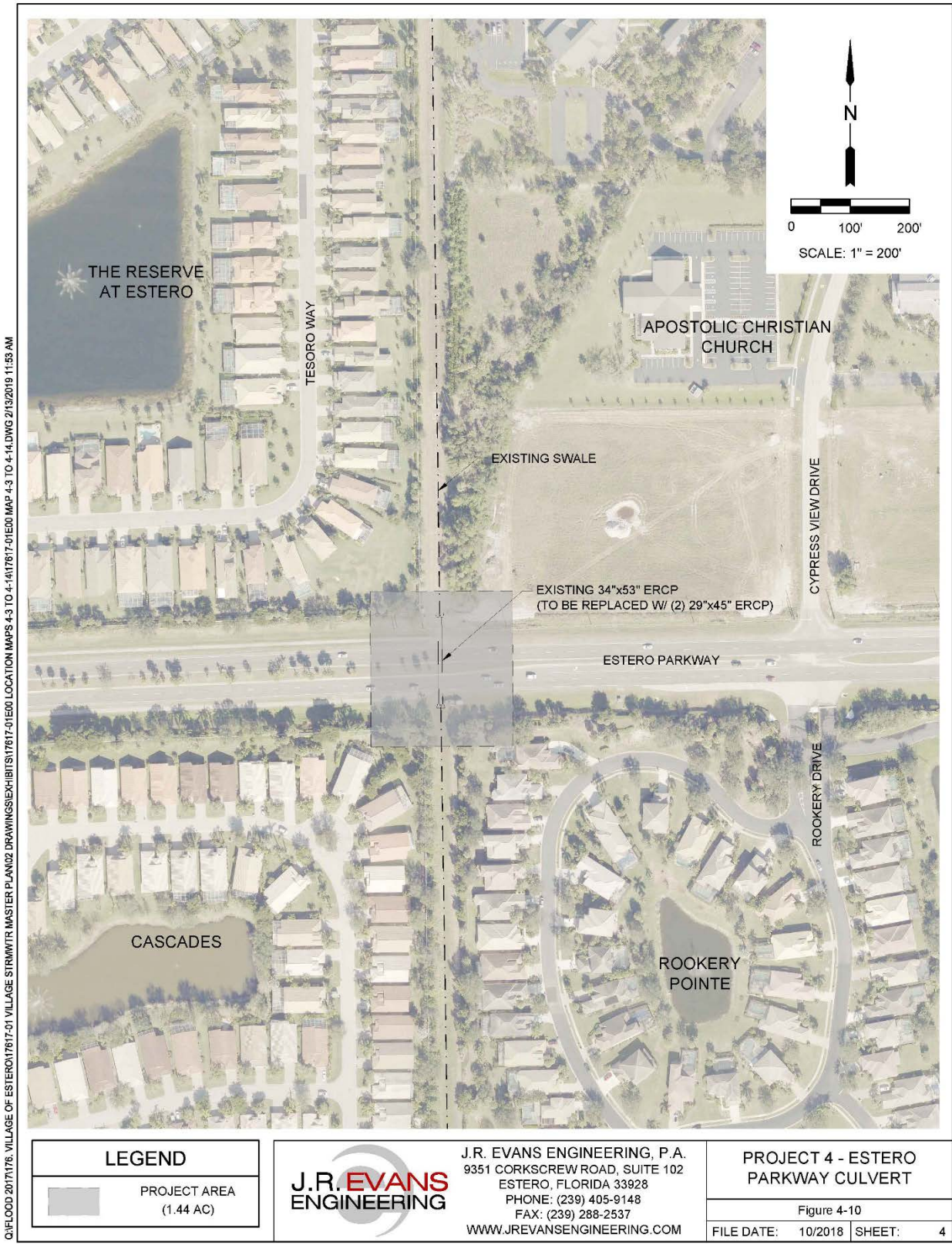
Figure 4-10: Project Four - Estero Pkwy Culvert Replacement
