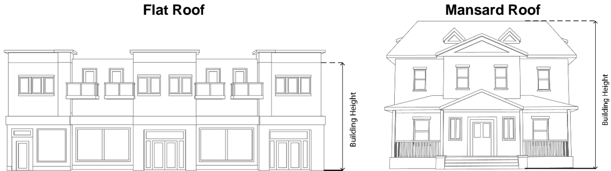
Figure 10-301.C-1: Flat and Mansard Roof Building Height Measurement
